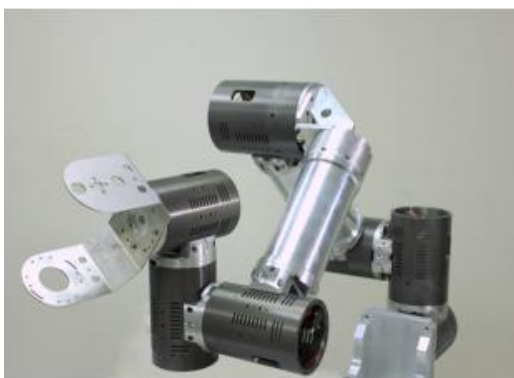
Fig. 1 The physical hardware assembly of the modularized 7-DoF manipulator with offsets at shoulder and wrist
